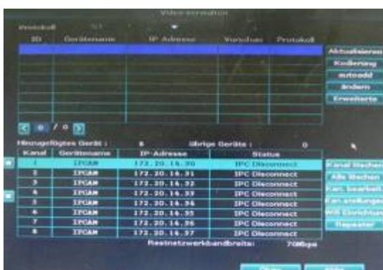
You can see the registered video cameras in the menu (right mouse button ◊ "Manage video"). As a rule, the available cameras registered in the recorder should already be displayed here.
